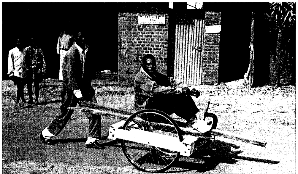
Joto Kasambala testing the prototype Mark la chassis with Patrick Chisi on board.
