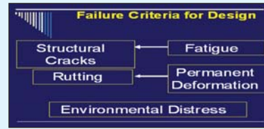
Fig. 2: Pavement Failure / Design Criteria
