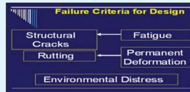
Fig. 2: Pavement Failure / Design Criteria
