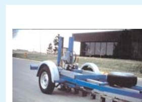
Photo 6: Pavement Evaluation Equipment (From FHWA)
